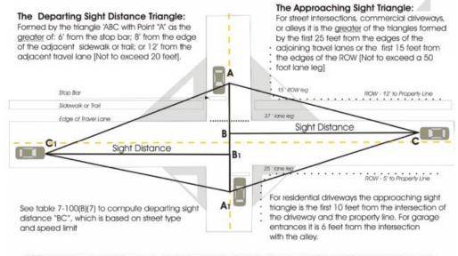
NOTE: All sight triangles prohibit objects or plants from obscuring visibility of objects between 3 ½ and 8 feet in height [accounting for vertical or horizontal ourves]. The departing sight distance triangle will apply to alleys, driveways and garage entrances - except that (where no ROW for additional lanes or tree planting strip is available) point % may be six (6)' from the edge of the adjacent sidewalk, trail or travel lane whichever is greater.
