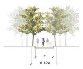
**D.** Surface Materials: Compact gravel, concrete, or asphalt or other material approved by the Administrator.
