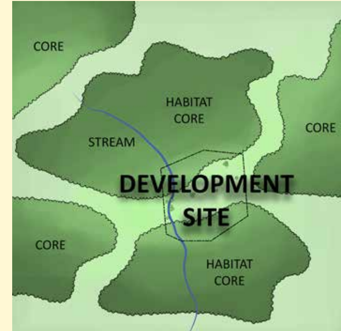
A development site in its larger context shows habitat cores and potential for increasing connectivity.
